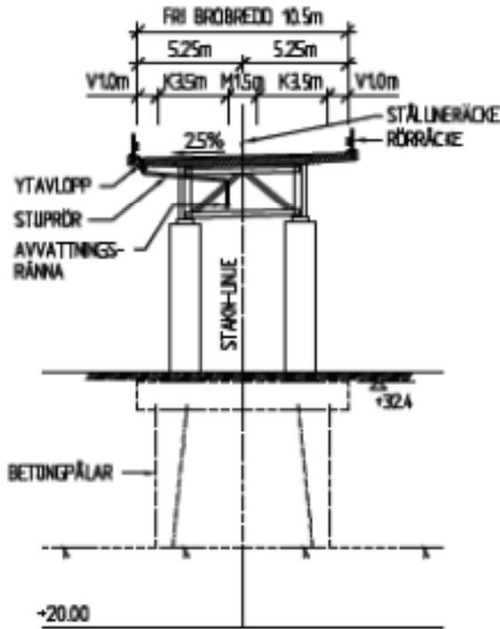
Figure 2.14. Cross-section of the studied bridge.
