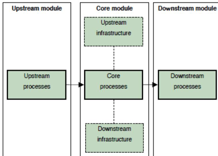
Figure 3.6. General system boundaries of construction project with Upstream and Downstream processes ( International EPD®System 2010).
