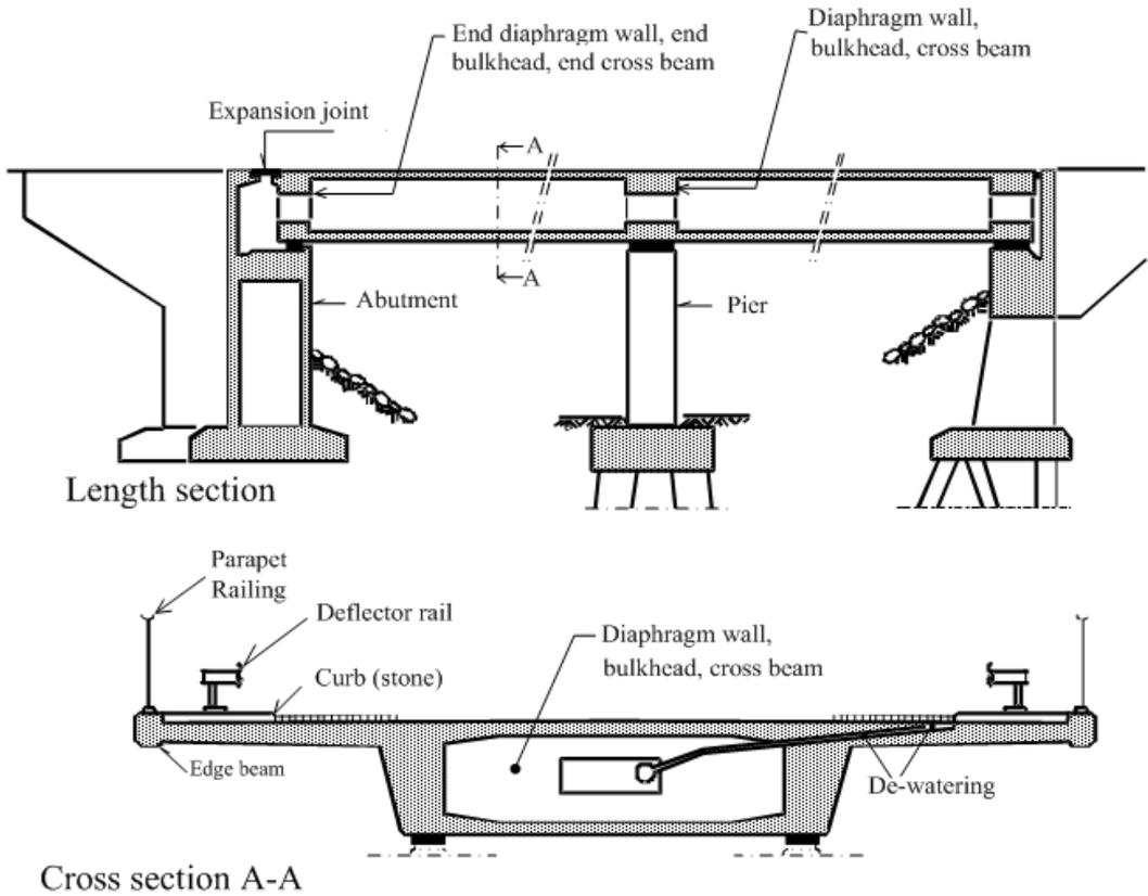
Figure 2.11. Notations in the longitudinal direction and in the cross direction for a typical box girder bridge with ordinary bearings and expansion joints.
