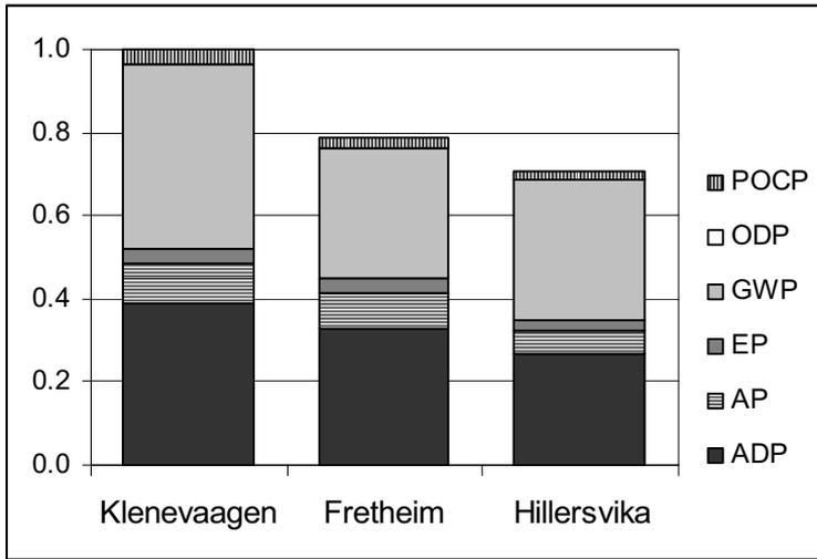
Figure 3.10. Total weighted impacts, relative to results for Klenevaagen Bridge (calculated on a per m<sup>2</sup> effective bridge area basis).
