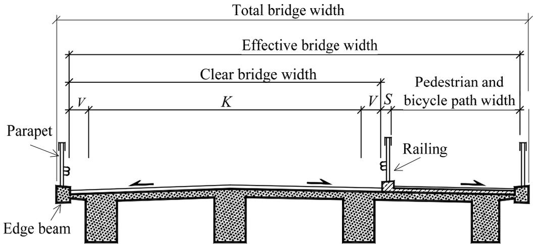
Figure 2.10. Notations and measures in cross direction of typical beam girder bridge carrying a roadway and a pedestrian and bicycle path.
