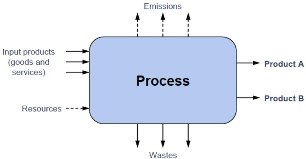
*Figure 3.5. Example of a multifunctional process, with several inputs, emissions and wastes, and providing two co-products A and B (Source: European Commission 2010b).*
