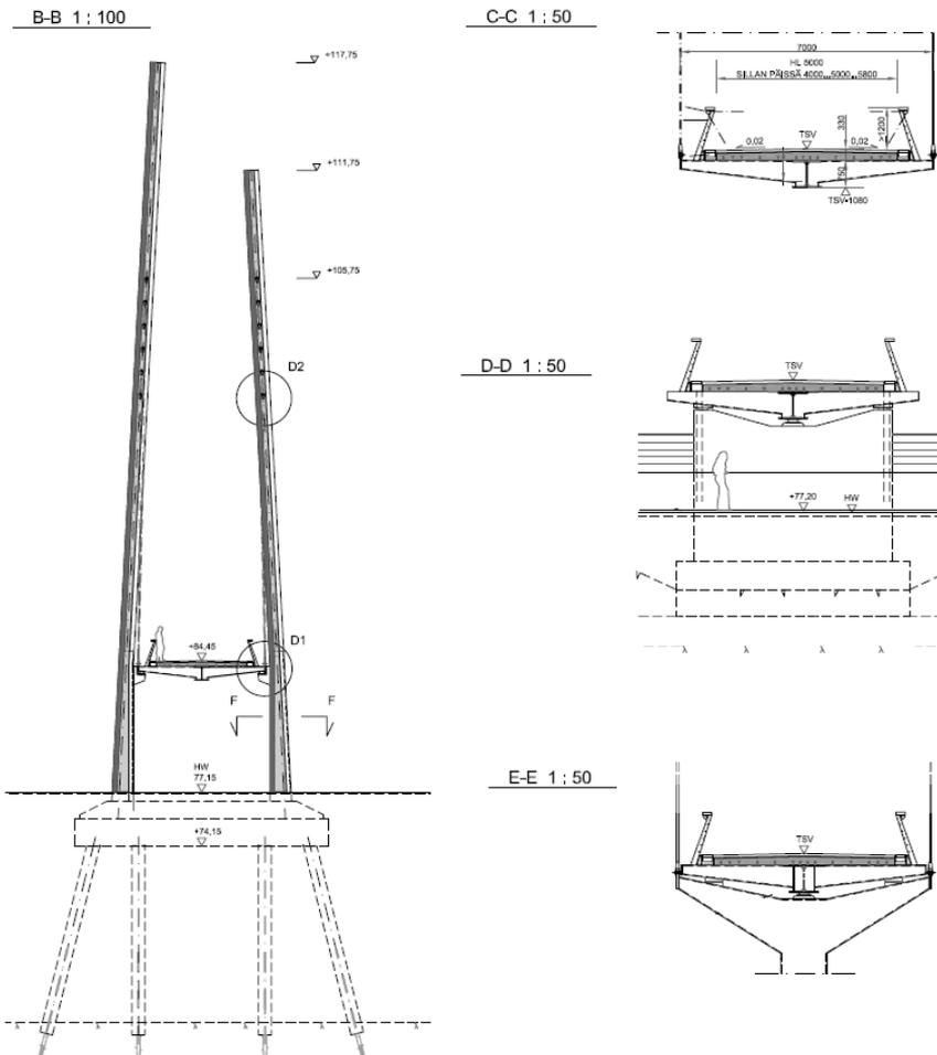
Figure 4.9. Cross-sections of Bridge No. 2.
