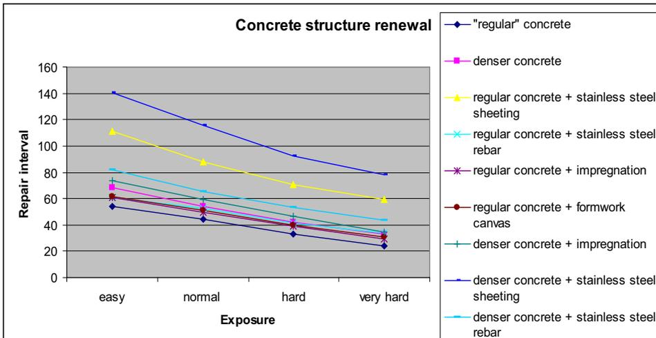
Figure 2; Concrete structure renewal for some alternatives
