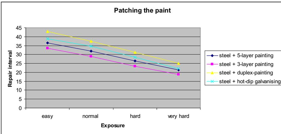
Figure 3; Patching the paint
