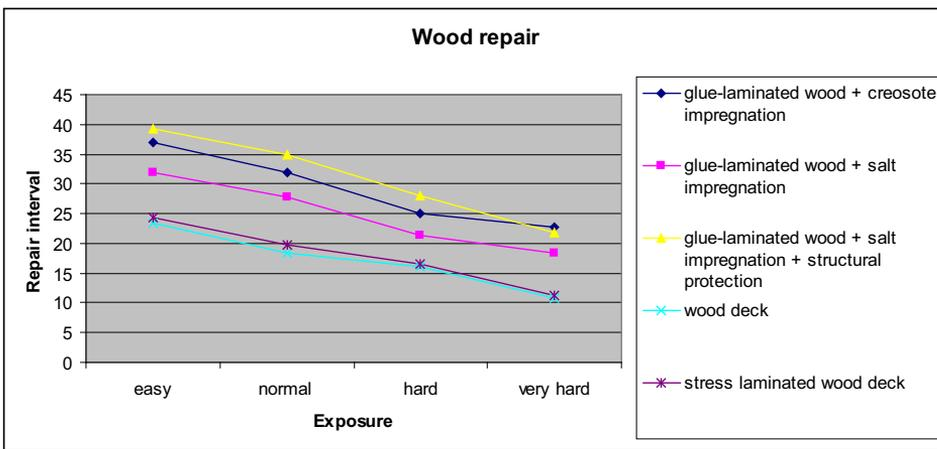
Figure 5; the repair of wooden member
