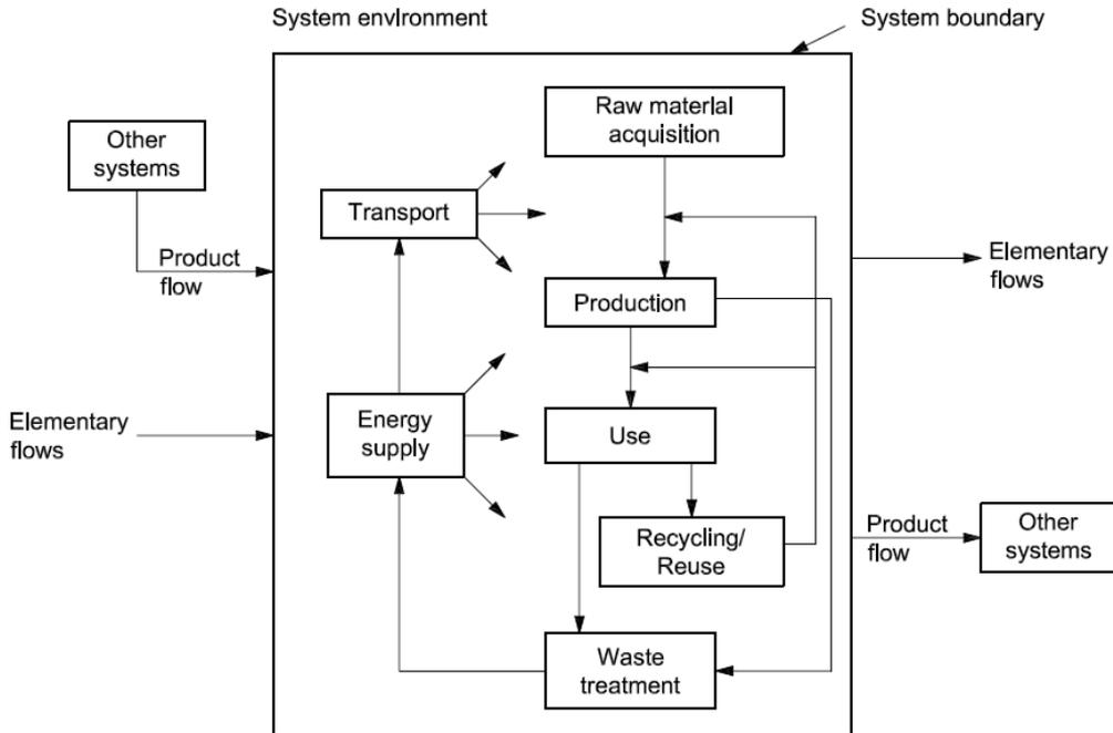
Figure 3.1. Illustration of a product system in LCA (ISO (2006a)).
