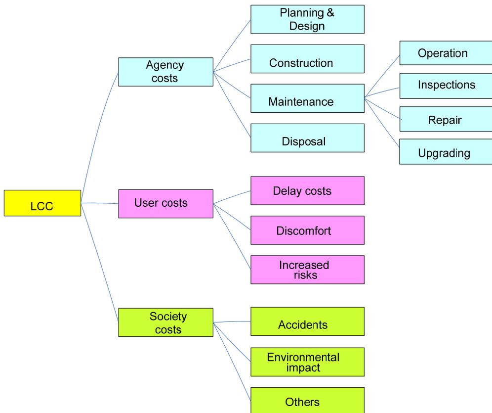
Figure 2.2. Schematic presentation of the different items in a complete LCC analysis.
