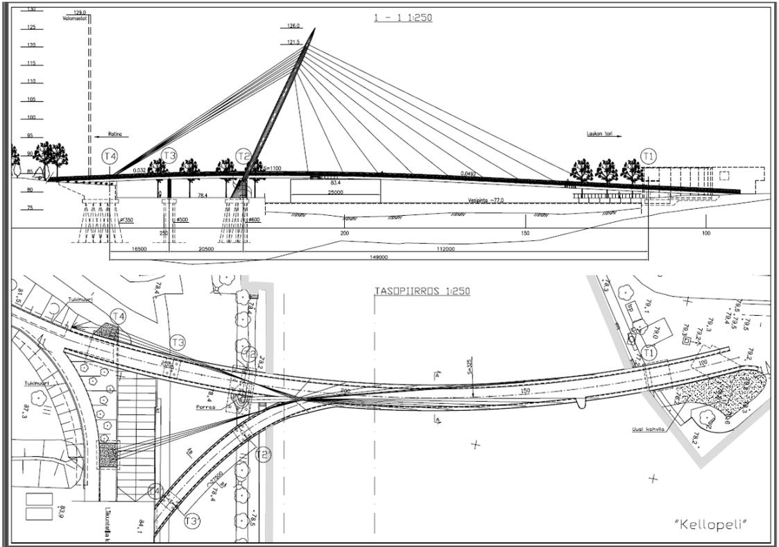
Figure 4.13. General drawing of Bridge No. 3.
