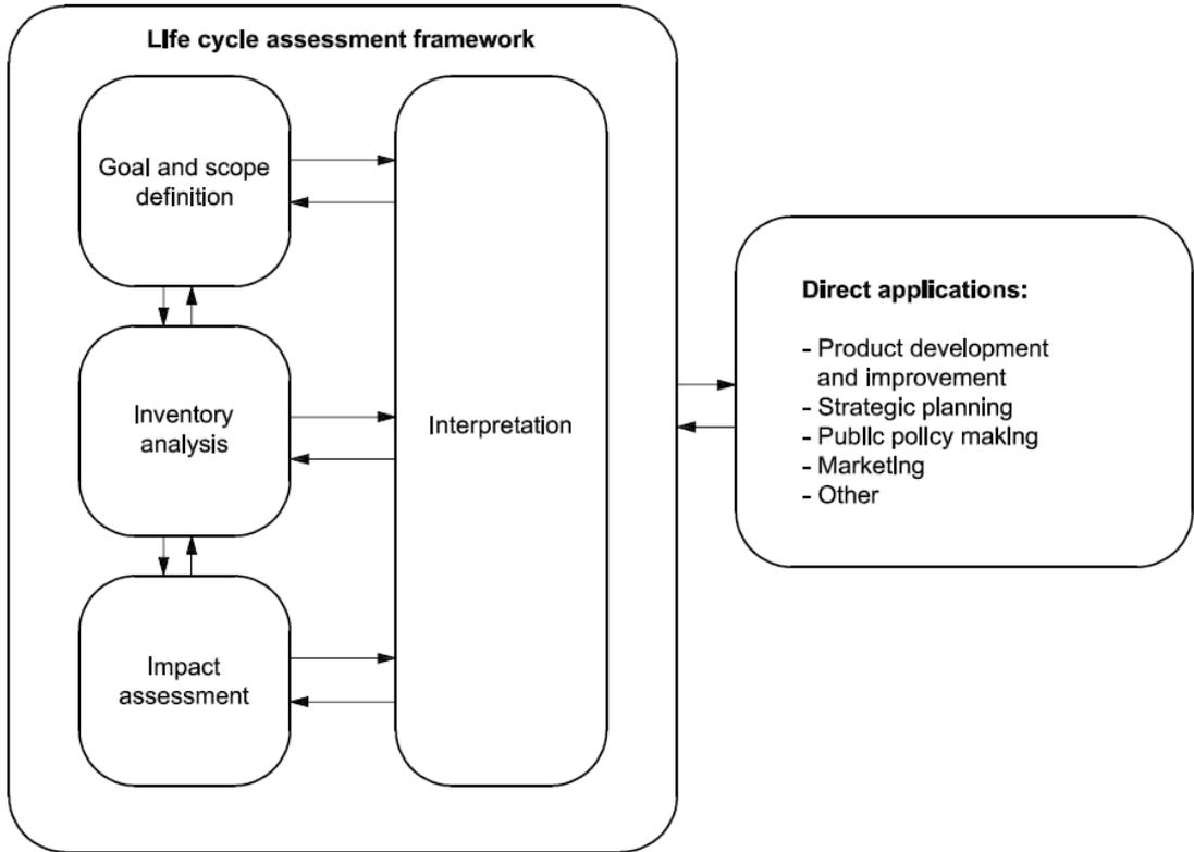
Figure 3.2. The four phases of LCA (ISO (2006a)).
