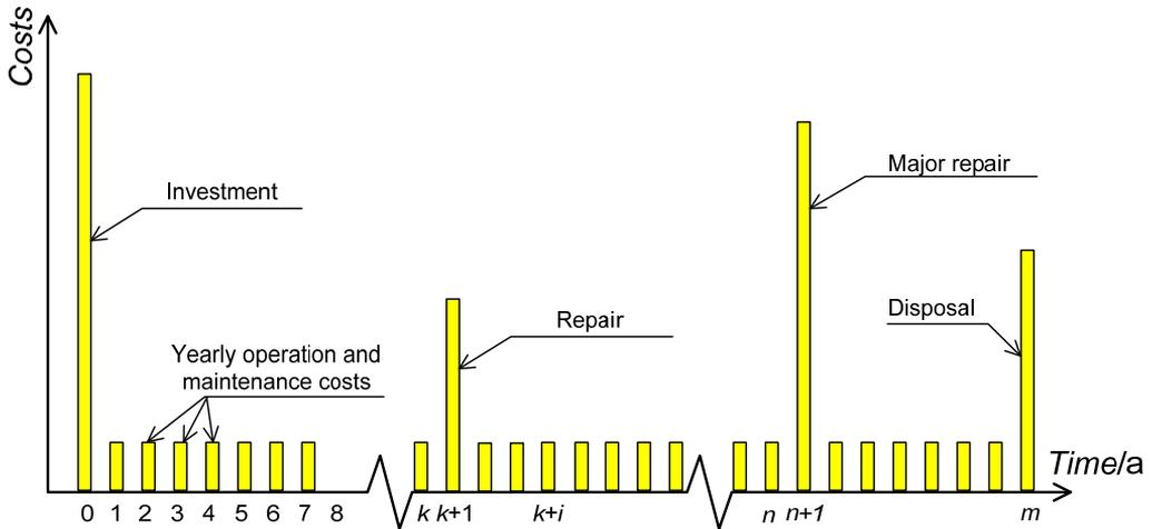
Figure 2.3. Schematical representation of agency costs for a bridge. The costs in this figure are not recalculated using the present value method.
