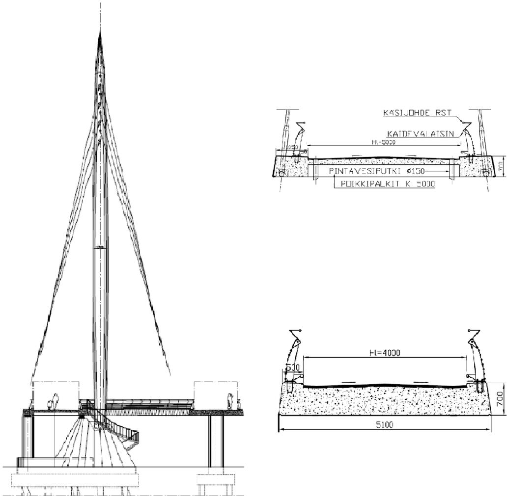
Figure 4.14. Longitudinal view and cross-sections of Bridge No. 3.
