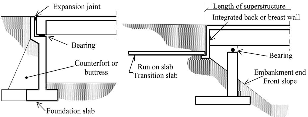
Figure 2.12. Notations for abutment elements in an ordinary bridge and in an integral bridge with integrated back walls.
