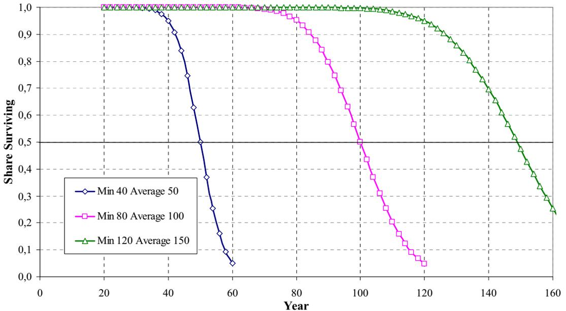
Figure 2.8. Requirement of standards for designing life-span of bridges. In Sweden the design life-span is defined as the lower 5% fractile of a distribution which can be assumed to be normally distributed.
