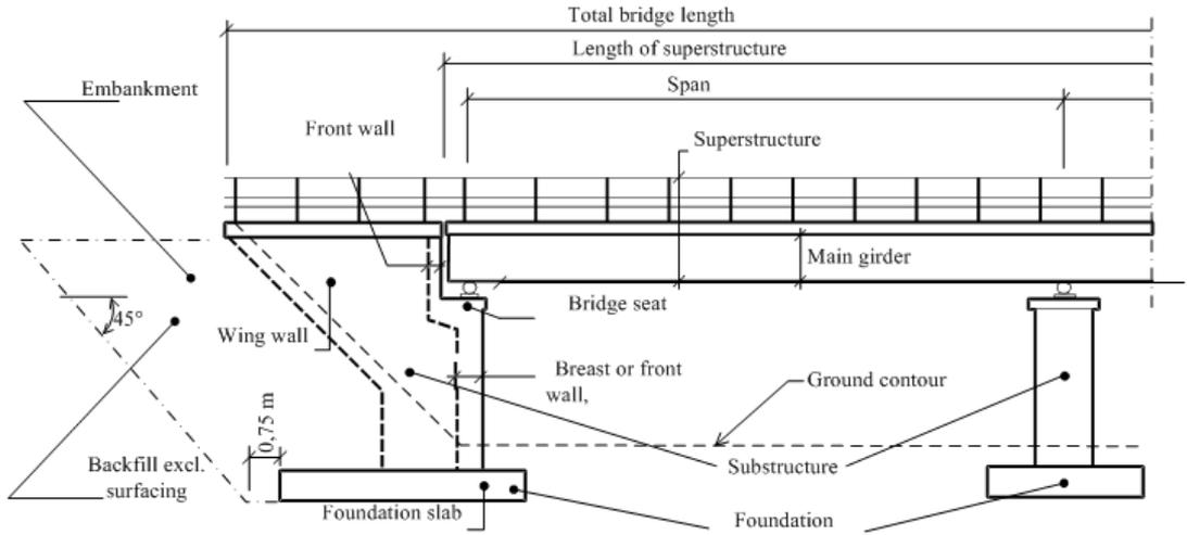
Figure 2.9. Notations and measures of a typical beam girder bridge with ordinary bearings and expansion joints.
