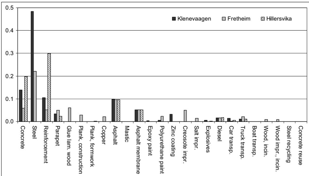
Figure 3.11. Total weighted impacts per functional unit, split up into input parameters.
