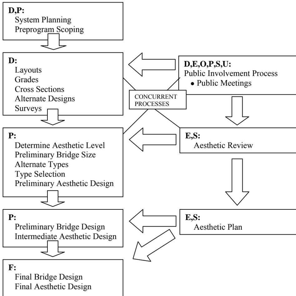
**Fig. 2.** Aesthetic design flow chart for Level B in the Minnesota Department of Transportation’s aesthetic design process. The key letters have the following meaning: D - district preliminary design, final design, maintenance and construction, E - environmental services, F - bridge design final, P - bridge design preliminary, S - site development, U - public, O - other agencies (State Historical Preservation Office, Dept. of Natural Resources, local government units, etc.).[1]
