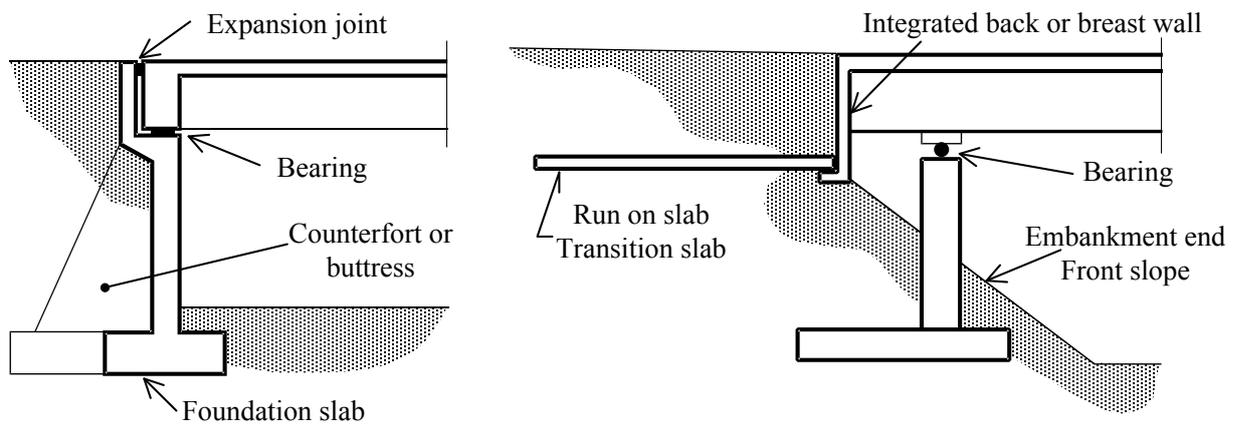
**Figure 4.4** Notations for abutment elements in an ordinary bridge and in an integral bridge with integrated back walls.
