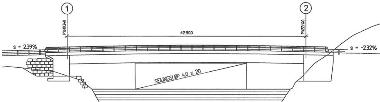
**Figure 6.1** Klenevågen Steel Box Girder Bridge has a bridge span of 42,8 m.
