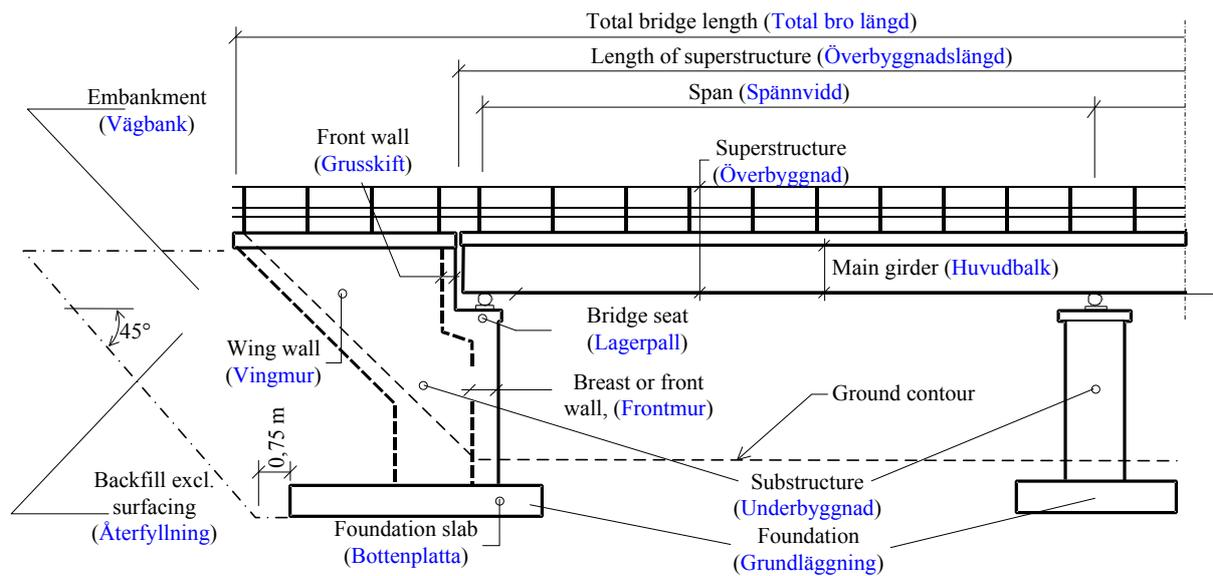
**Figure 4.1** Notations and measures of a typical beam girder bridge with ordinary bearings and expansion joints.
