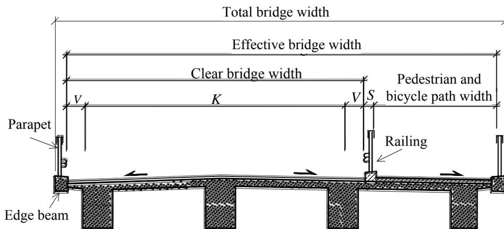
**Figure 4.2** Notations and measures in cross direction of typical beam girder bridge carrying a roadway and a pedestrian and bicycle path.
