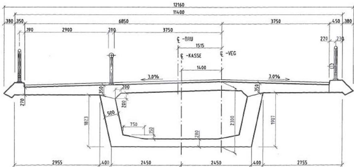
**Figure 6.6** Hillersvika Concrete Box Girder Bridge has an effective bridge width of 10,6 m.
