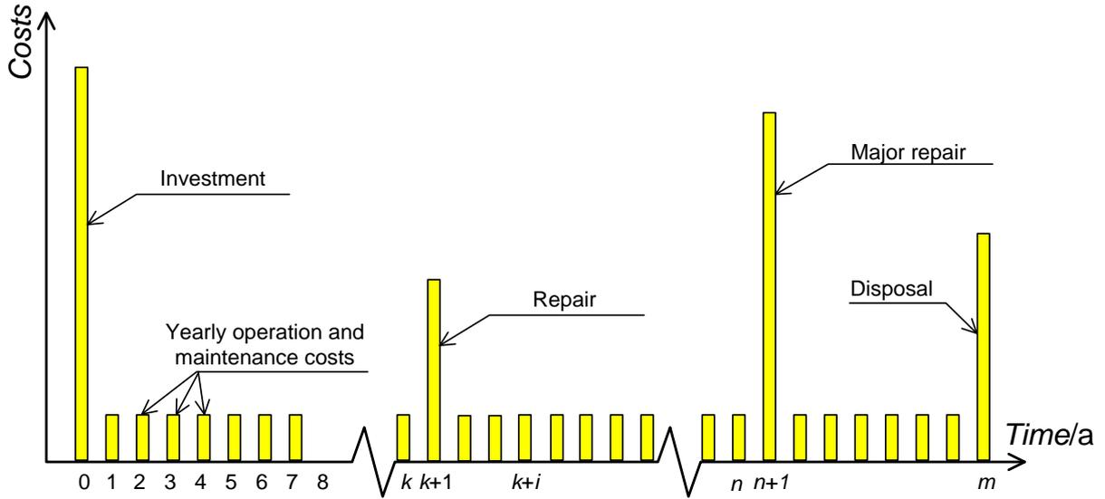
**Figure 3.3** Schematically representation of agency costs for a bridge. The costs in this figure are not recalculated using the present value method.
