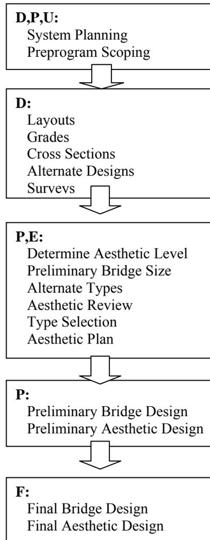
**Fig. 3.** Aesthetic design flow chart for Level C in the Minnesota Department of Transportation's aesthetic design process. The key letters have the following meaning: *D* - district preliminary design, final design, maintenance and construction, *E* - environmental services, *F* - bridge design final, *P* - bridge design preliminary, *S* - site development, *U* - public. [1]
