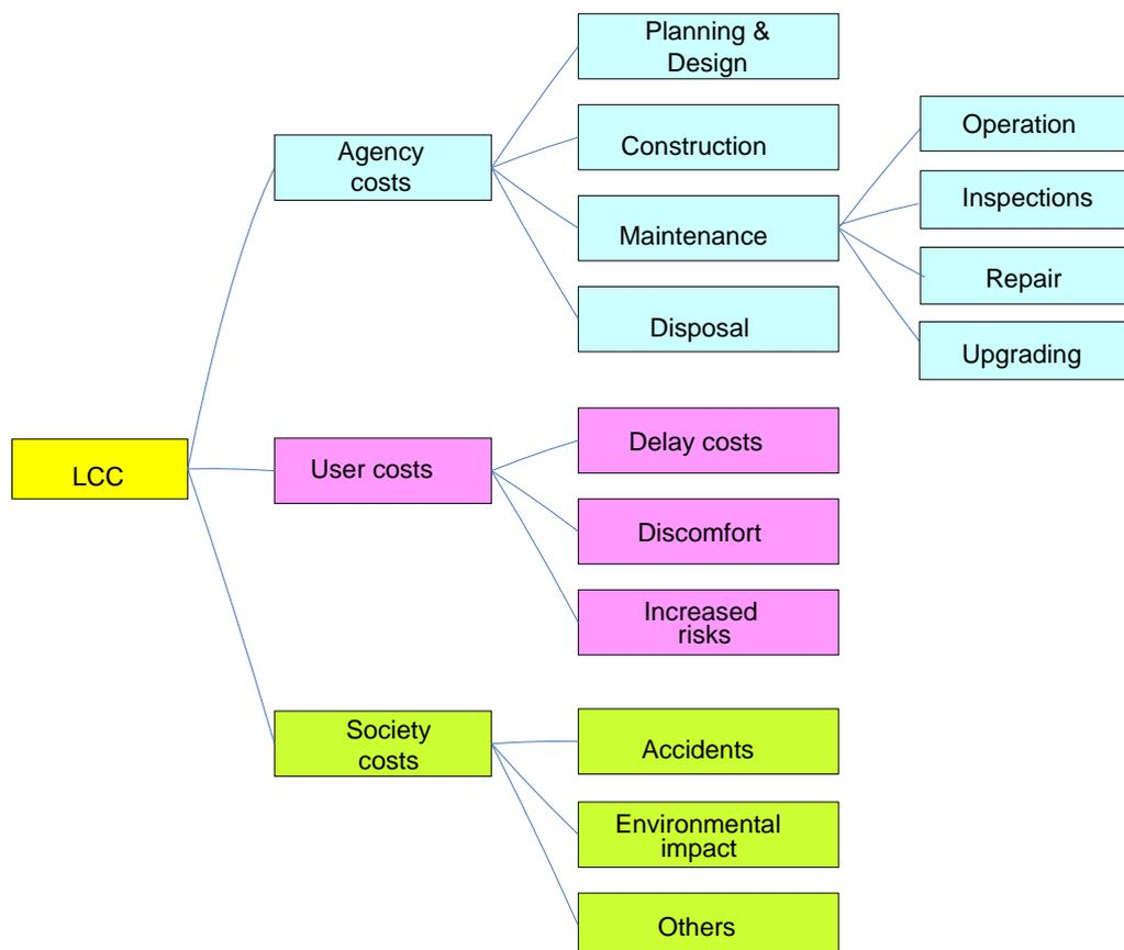
**Figure 3.2** Schematic presentation of the different items in a complete LCC analysis.
