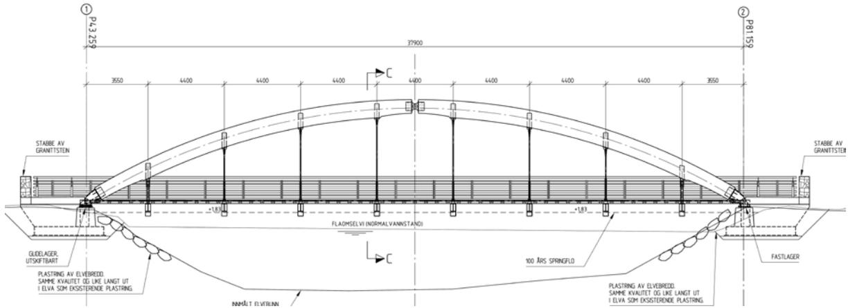
Figure 6.3 Fretheim Timber Arch Bridge has a bridge span of 37,9 m.
