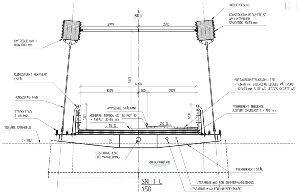
Figure 6.4 Fretheim Timber Arch Bridge has an effective bridge width of 6,05 m.
