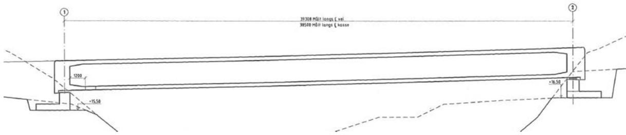
**Figure 6.5** Hillersvika Concrete Box Girder Bridge has a bridge span of 39,3 m.
