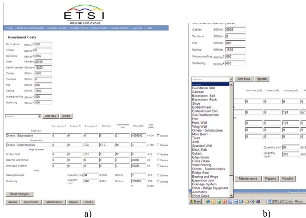
Figure 5.5 Page 4, the investments menu. A large amount of different bridge parts can be added and modified.
