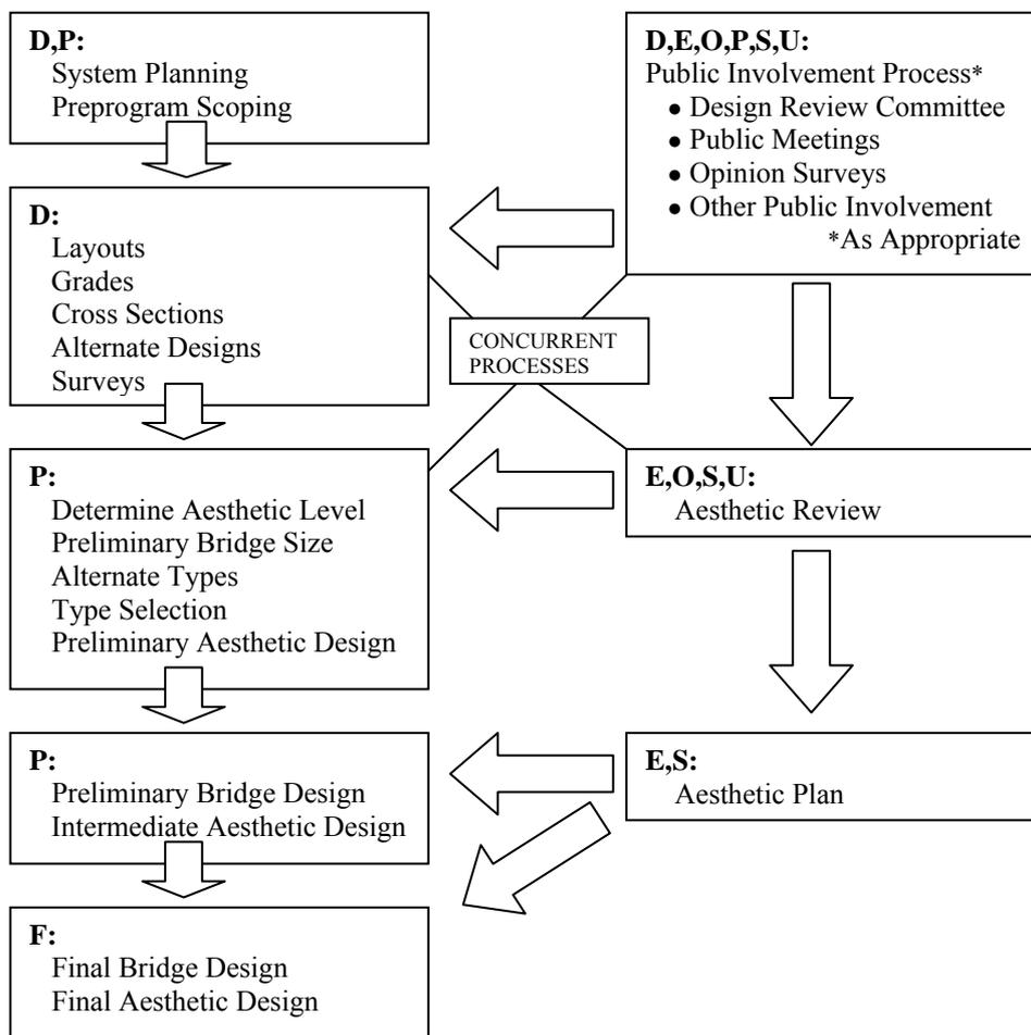
**Fig. 1.** Aesthetic design flow chart for Level A in the Minnesota Department of Transportation’s aesthetic design process. The key letters have the following meaning: D - district preliminary design, final design, maintenance and construction, E - environmental services, F - bridge design final, P - bridge design preliminary, S - site development, U - public, O - other agencies (State Historical Preservation Office, Dept. of Natural Resources, local government units, etc.).[1]
