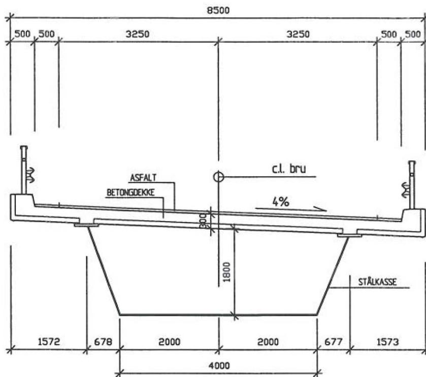
**Figure 6.2** Klenevågen Steel Box Girder Bridge has an effective bridge width of 7,5 m.
