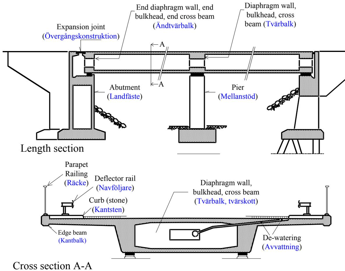
**Figure 4.3** Notations in the longitudinal direction and in the cross direction for a typical box girder bridge with ordinary bearings and expansion joints.
